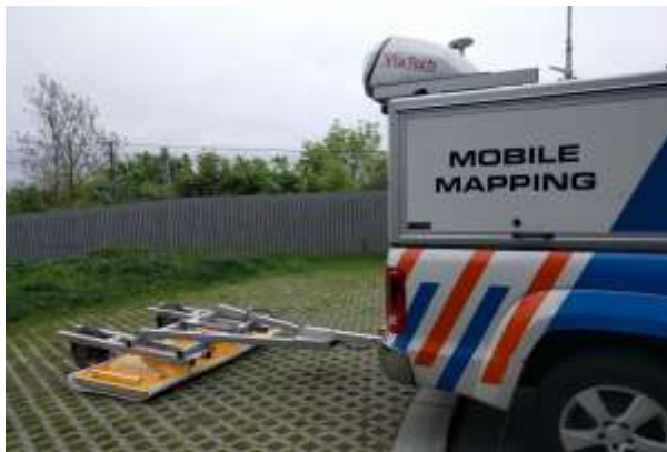
Markpenetrerande radar (GeoScopeTM GPR)
